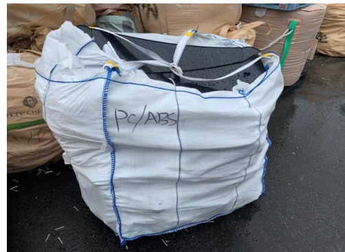
Plastic blending different type of polymers, so-called "polymer-alloy", (e.g., PC/ABS)
