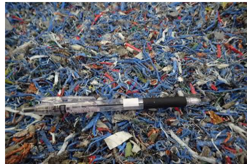
PVC cable (shredded)
